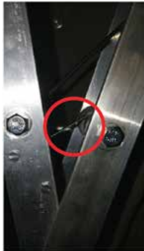
Location of Limit Switch on the arm
